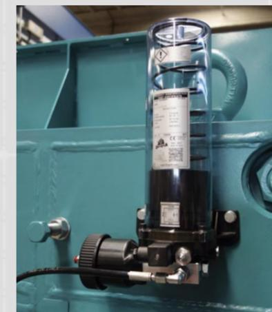
Automatic timed lubrication system designed to guarantee long life and perfect efficiency of all moving elements.
