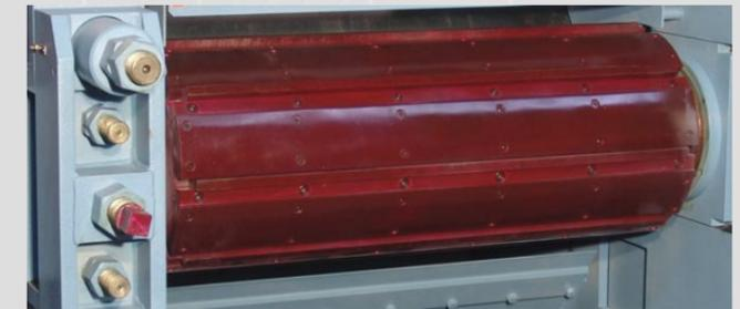
Fast cylinder equipped with interchangeable anti-wearing steel blades and exchangeable linings to protect the shaft.
